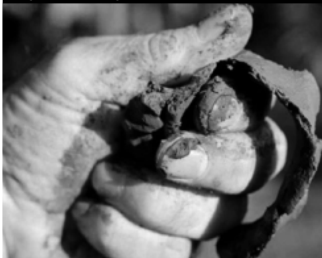
Figure 1: Making a soil ribbon
