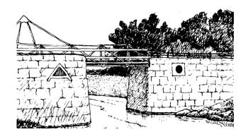
Parks Canada staff at the Lockstation open the bridge by turning a crank in the pivot of the bridge. Counter weights and a set of roller wheels mounted on a circular track underneath allow the bridge to be swung open with little effort. The opening of the bridge is both a unique experience to watch and a fixture in Burritt's Rapids life during boating season.
